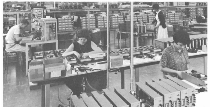
Main production area is neat, well organized. Power supplies made here convert power from AC to DC for operating other electronic units.
